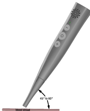
Figure 2 – VascuChek™ is typically held between 45° and 60° relative to the vessel being tested.
